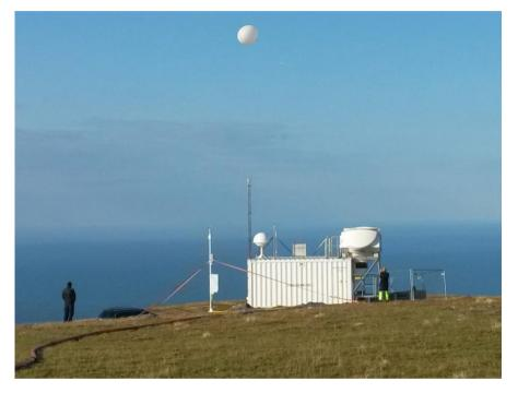
Upper air soundings are essential for a complete atmospheric weather profile that enables accurate forecasting. Manually operating sounding stations in remote locations is difficult and expensive, however, especially during harsh weather.
