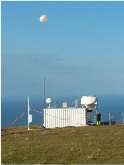
Vaisala Automatic Sounding Station AUTOSONDE AS41 is an upper-air observation system for synoptic and adaptive use. With a loading capacity of 60 radiosondes, it provides the longest autonomous sounding capacity on the market.
