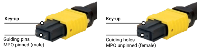
Figure 1. MPO and MTP male and female connectors
