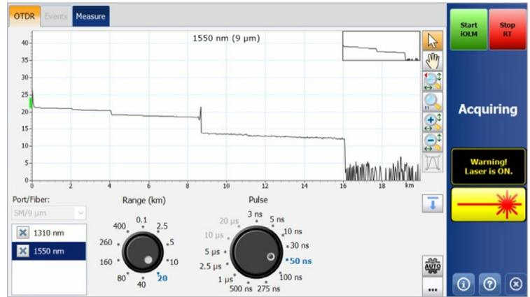
*Dialing wheels allows to adjust real time acquisition parameters on the fly, immediately seeing the effect on the trace for optimal efficiency. Ready to launch the characterization? Just press the "start iOLM" button, no need to manually interrupt real time nor getting into any menus.*
