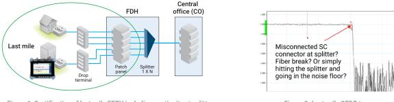
Figure 1. Certification of last-mile FTTH including continuity at splitter.
