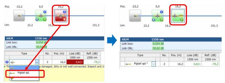
When you change events from a regular connector (threshold at 0.5 db in the example above) to a custom "pigtail spliced connector," a custom-built icon appears and the unit adjusts to a custom threshold (0.75 db in the example above) so you can avoid false failures. Modified elements are tagged with an asterisk (\*) for traceability.
