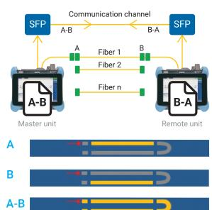
Using the loopback test method and iLOOP option on your iOLM enables you to test two fibers at once. View only the A link, B link, or the complete A-B link including the loop.
