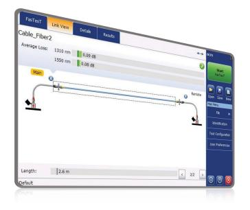
Multifunction optical loss test set (OLTS) measuring insertion loss (IL), optical return loss (ORL) and fiber length at two wavelengths in 5 seconds via fully automated bidirectional FasTesT™ analysis.
