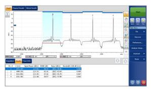
The FTBx-5235 displays channel power, channel wavelength and OSNR. Above: example of CWDM network OSA display. Below: example of DWDM network OSA display.
