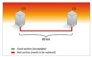
Traditional PMD measurement techniques provide a total link PMD value, but do not provide insight into which spans are causing the link to fail the test.
