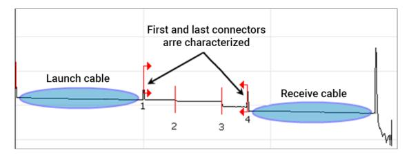
Note: To measure the loss in the first connector with the SPSB-EF launch cable, the OTDR pulse width should be 100 ns or shorter and the connection to the OTDR port should have a relfection value of -45 dB or better. A 50 µm test link must also be selected.
