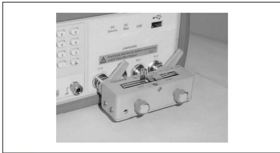
Figure 7-19 Connecting a shorting bar
