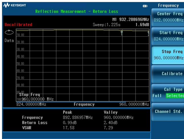
Figure 5. Reflection measurement mode waiting for OSL calibration
