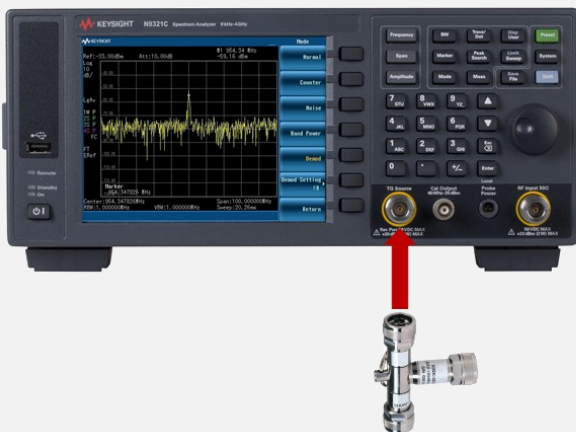
Figure 6. Performing open-short-load calibration on the N9322C BSA
