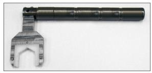
Figure 9. Bent torque wrench
