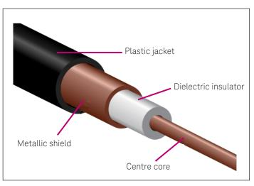
Figure 10. Coaxial cable cross section
