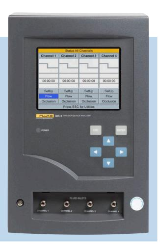
Ensure infusion pumps are tested accurately and quickly with the IDA-5 Infusion Device Analyzer. The IDA-5 is based on sophisticated measurement technology trusted by biomedical professionals around the world for over 20 years. The IDA-5 is a full-featured device that measures instantaneous flow, average flow, occlusion pressure and dual flow based on IEC60601-2-24.
