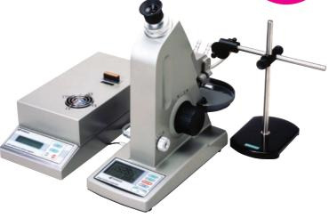
matching the boundary line at the intersection point of the cross hairs. These refractometers can be connected to the digital printer. The DR-M4 is a high refractive index version of the DR-M2, with a refractive index measurement range of 1.4700 to 1.8700 (at a wavelength of 589nm). The DR-M4 shares common appearance and features with the DR-M2.
