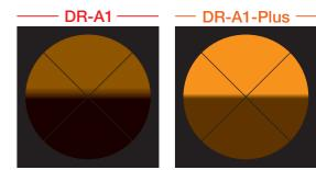
The DR-A1 has a slightly dimmer field of view, which makes it difficult to measure emulsions or dark samples.
