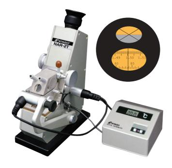
Designed for use with compounds that require measurement at high temperatures (up to 120°C). Capable of measuring samples from 5 to 120°C, such as substances with a melting point higher than room temperature, or compounds containing substances with a transition temperature below 120°C. Aside from liquid samples, glass, films, plastics and other solid samples can also be measured.
