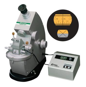
The NAR-3T is the unit with the highest degree of precision and accuracy among the Abbe Refractometers. It was developed to give improved measurement accuracy and ease of use. This was achieved by making fundamental improvements to the optical system and utilizing a larger scale, which allows for a refractive index scale measurements of up to 0.00005. Incorporating a high intensity lamp and using a double control knob gives quick and more accurate control
