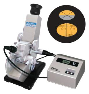
The NAR-1T LIQUID is for liquid sample measurement only. This model has the Refractive Index scale and Brix scale, and operates with D line (589nm) light source. Calibration is performed using distilled water.
