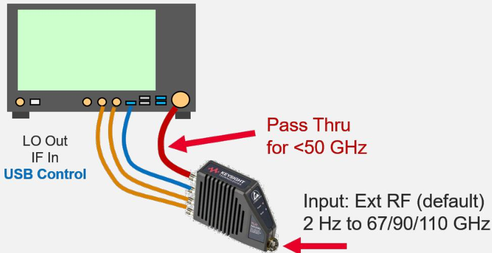
Figure 6. Configuration 1, single input.
