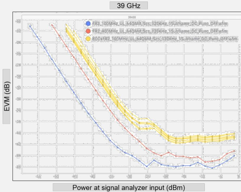
Figure 5. FR2, 39 GHz carrier, CP-OFDM Uplink, 1x100 MHz (blue) and 1x400 MHz (red) and 8x100 MHz (yellow), 64 QAM, 120 kHz SCS, phase tracking on
