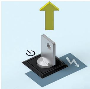
The key switch is locked and high-voltage preparation is not possible. When locked, the key can be removed and the system secured against unauthorised high-voltage operation.
