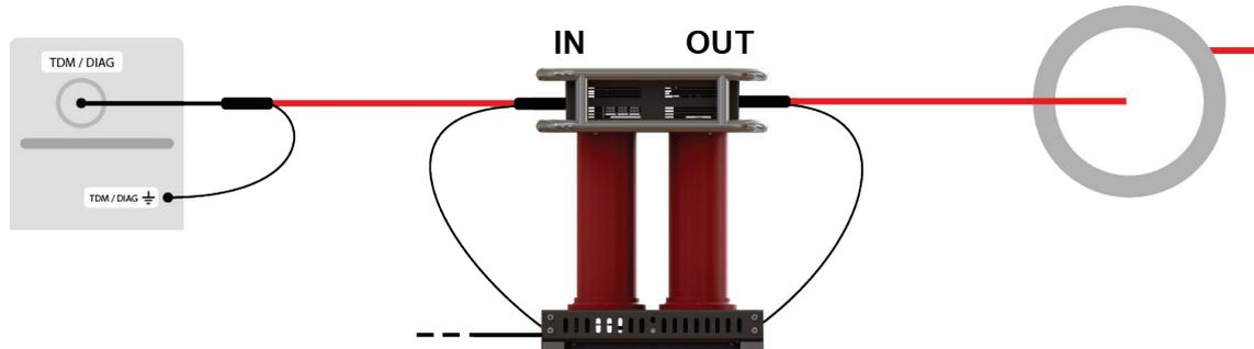
In all other operating modes, the partial discharge coupler must be disconnected from the HV path. The HV connection cable connected to the input ("IN") remains connected to the coupler and is earthed via the two parking sockets.
