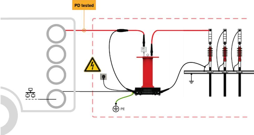
PD diagnostics with internal PD coupler PDS 60 or PDS 60-HP
