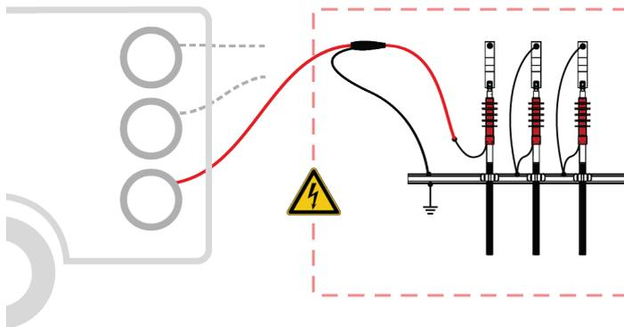
Cable shield must not be earthed at both ends of the cable!
