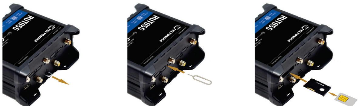
After the new SIM card is inserted in the orientation shown, the holder must be pushed back into the slot until it clicks into place. Following the installation of a new SIM card, the PIN of the SIM card must be stored and the configuration of the access point (APN) adjusted.
