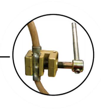
4. Secure the cable drum brake again.
