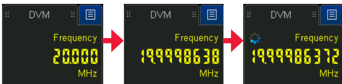
Figure 33. The precise 10-digit counter found the true frequency of a clock to be a little less than 20 MHz.
