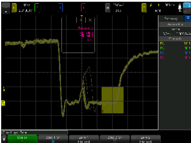
Figure 12. Hardware zone triggers immediately.
