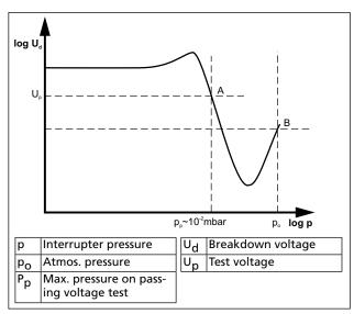
Flashover threshold voltage plotted against pressure in vacuum chamber.
