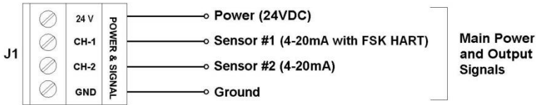
Figure A - 6 Power and Signal Connector J1 on HART Supported TRANS-2
