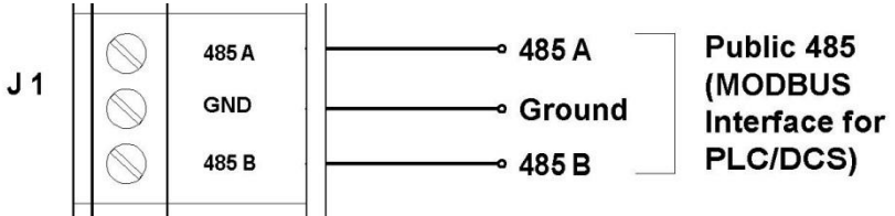
Figure 4-9 Wiring Diagram for the ModBus Interface
