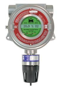
Detcon Model DM-634 sensors are non-intrusive "Smart" sensors designed to monitor ambient air for concentrations of Oxygen in the range 0-25% by volume. The sensor assembly consists of a sensor in a stainless steel housing that includes a splashguard with integral cal port, a plug-in control transmitter circuit, a base connector board and an explosion proof enclosure.
