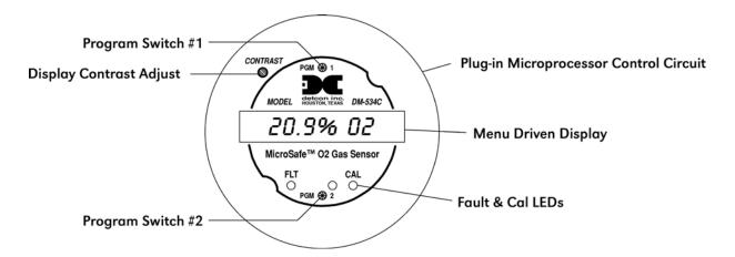
**Figure 2 Microprocessor Control Circuit**
