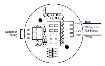
Figure 8 Sensor Connector PCB
