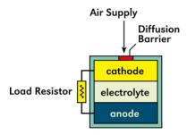
Figure 1 Construction of Galvanic Cell
