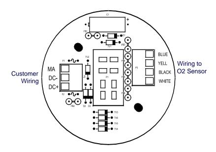
Figure 3 Base connector board
