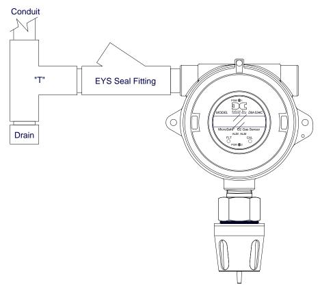
Figure 6 Typical Installation
