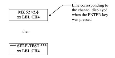
The user can interrupt the self-test cycle before it is completed by pressing the ACKNOWLEDGEMENT key.
