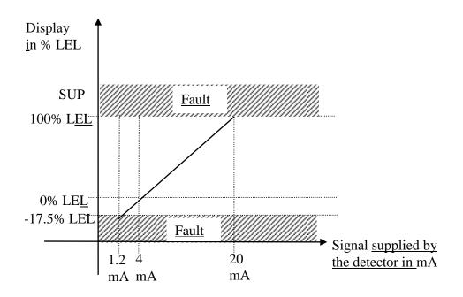
**<u>Please note</u>**: When the value measured is  $\geq 100\%$  LEL, the measuring device memorises the fact that the value has exceeded the scale and the channels switch to alarm and fault mode. Resetting these statuses is a manual operation to be performed by the user, who must follow the safety regulations specific to the site. The reset is checked either by turning the device on and off or by a maintenance inspection.
