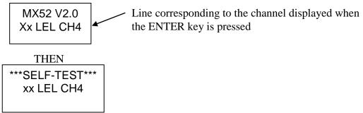
The user can be stop the self-test cycle early by pressing the CLEAR key.
