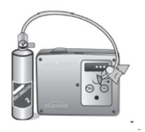
At this point all on-board and remote alarms should be activated and the 4-20 mA signal should reflect the display reading on the instruments.
