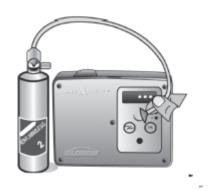
With the "zero" gas still flowing to the sensor, press and hold the key for a total of 10 seconds. During the first 5 seconds the normal screen is still displayed. During the next 5 seconds, the text or numeric display flashes once per second. If the key is still held after the full 10 seconds the word "ZERO" is displayed.
